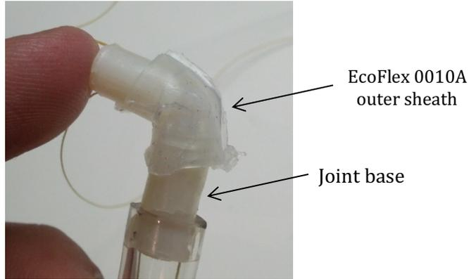
**Figure 29. 2:1 scale pin joint prototype**
