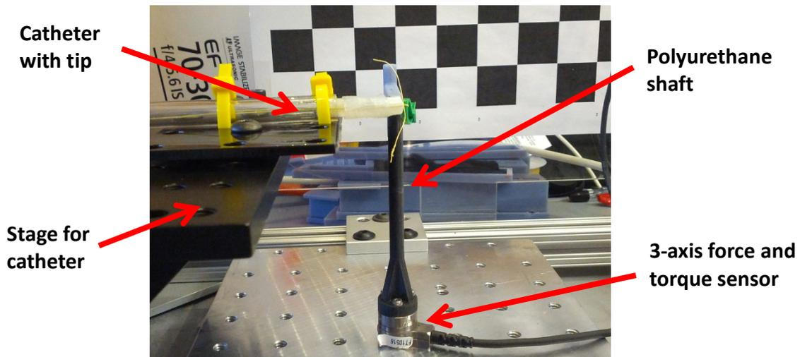
**Figure 30. Force testing setup, with components highlighted**
