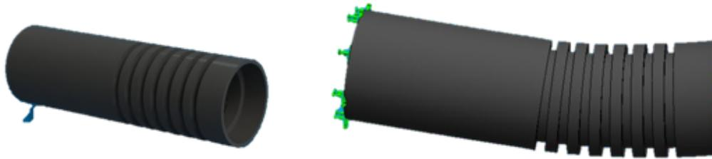
**Figure 21. CAD model of bellows joint catheter.**
