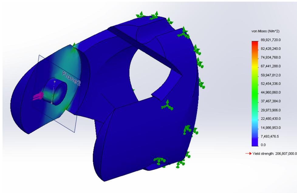
**Figure 12. CAD model of 1N force on pin in direction of arrow shown**
