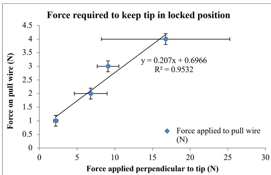
**Figure 33. Force required to keep tip in locked position**
