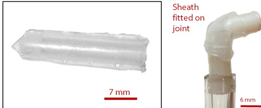
**Figure 10. Image of molded sheath made from Ecoflex 0010A silicone rubber pre-trimming (left); catheter with inelastic and elastic sheath fitted on joint (right)**
