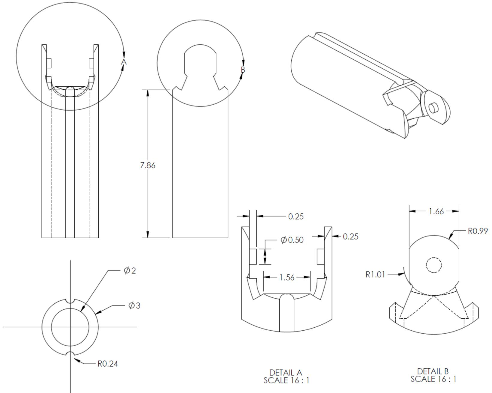
Figure 36. Bottom part of pin joint
