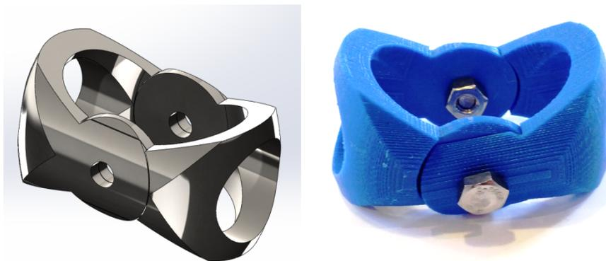
**Figure 25. Second prototype CAD model (left) and 15:1 scale 3D printed joint (right)**
