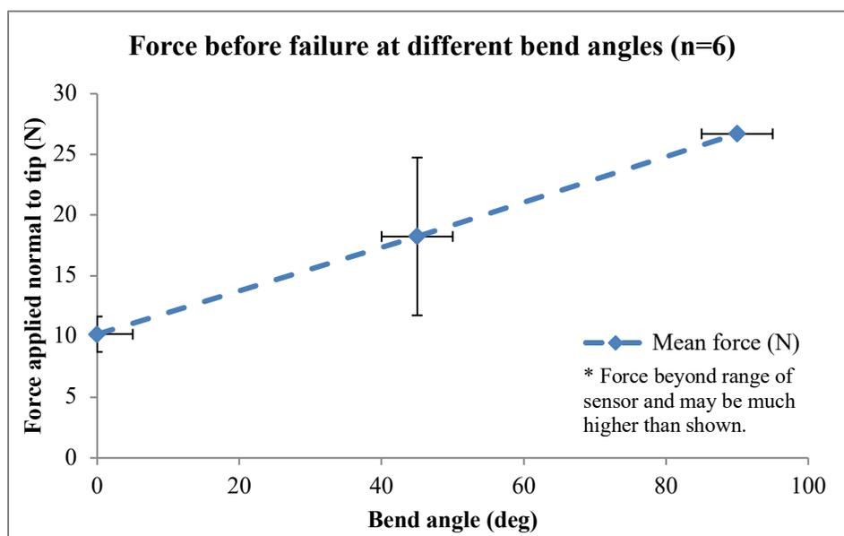
**Figure 32. Force before failure at different bend angles**
