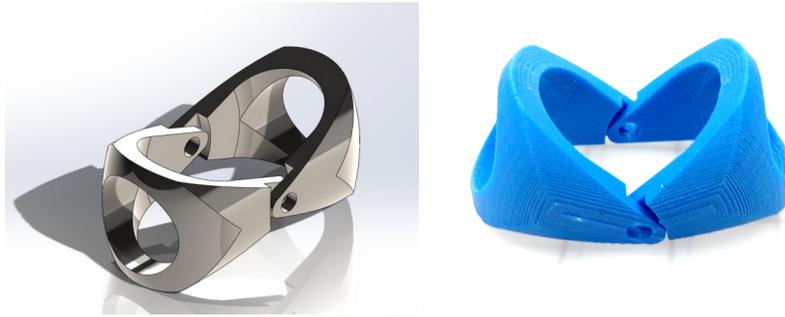
**Figure 24. First prototype CAD model (left) and 15:1 scale 3D printed joint (right)**
