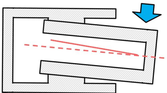
**Figure 15. Lateral force applied to tip of catheter**
