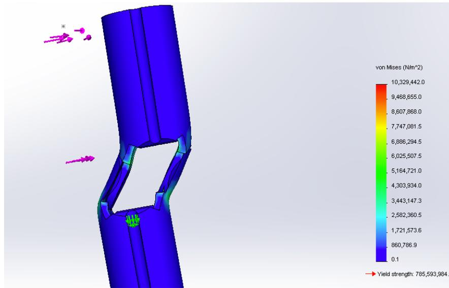
**Figure 16. CAD model of 1N lateral force distributed over entire top section of the catheter joint**
