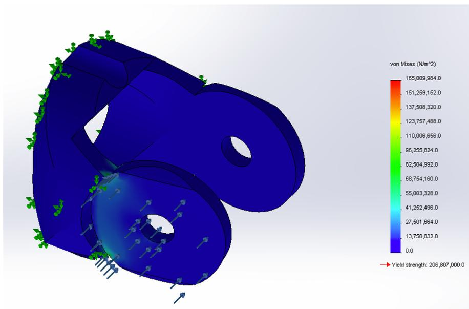
**Figure 14. CAD model of  $\frac{1}{2}$  N force over the articular surface of the inner socket**
