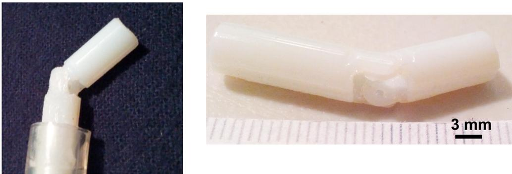
**Figure 9. Assembled catheter joint before addition of pull wires and outer sheath (left); close-up view of catheter joint (right)**
