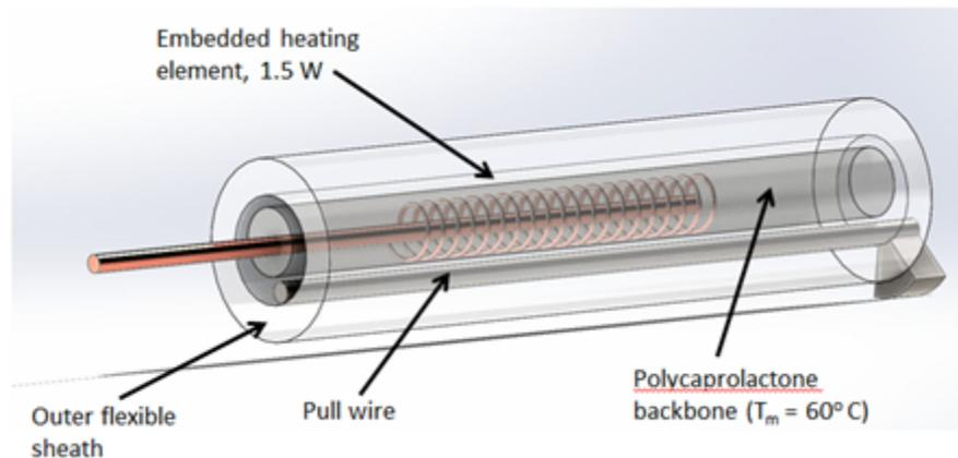
**Figure 22. CAD model of thermoplastic catheter backbone inside a catheter lumen**
