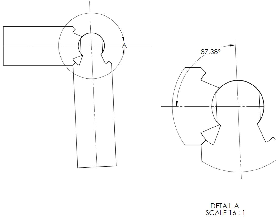
**Figure 38. Pin joint assembly**
