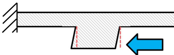
Figure 11. Shear loading on pin
