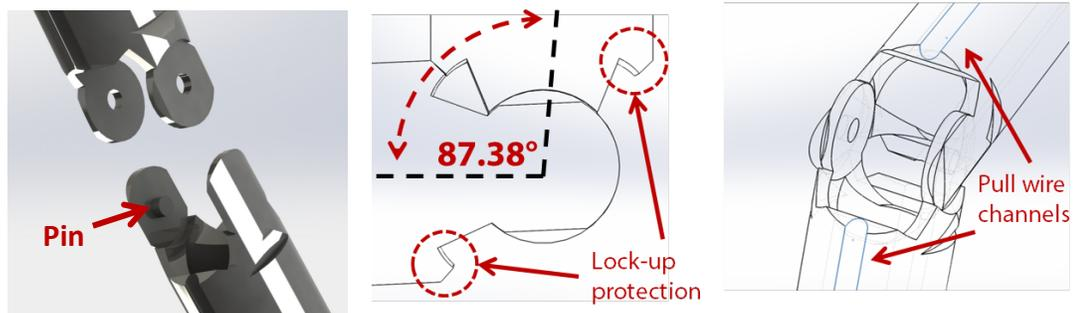
**Figure 8. Exploded view of the top and bottom portions of the catheter joint, with the pin highlighted (left); the maximum theoretical bend angle of the catheter as a result of a lock-up protection mechanism (center); pull wire channels integrated into the catheter lumen (right)**
