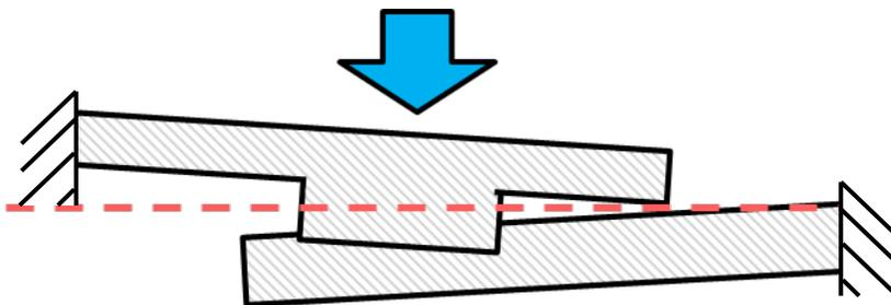
**Figure 13. Crushing of joint**
