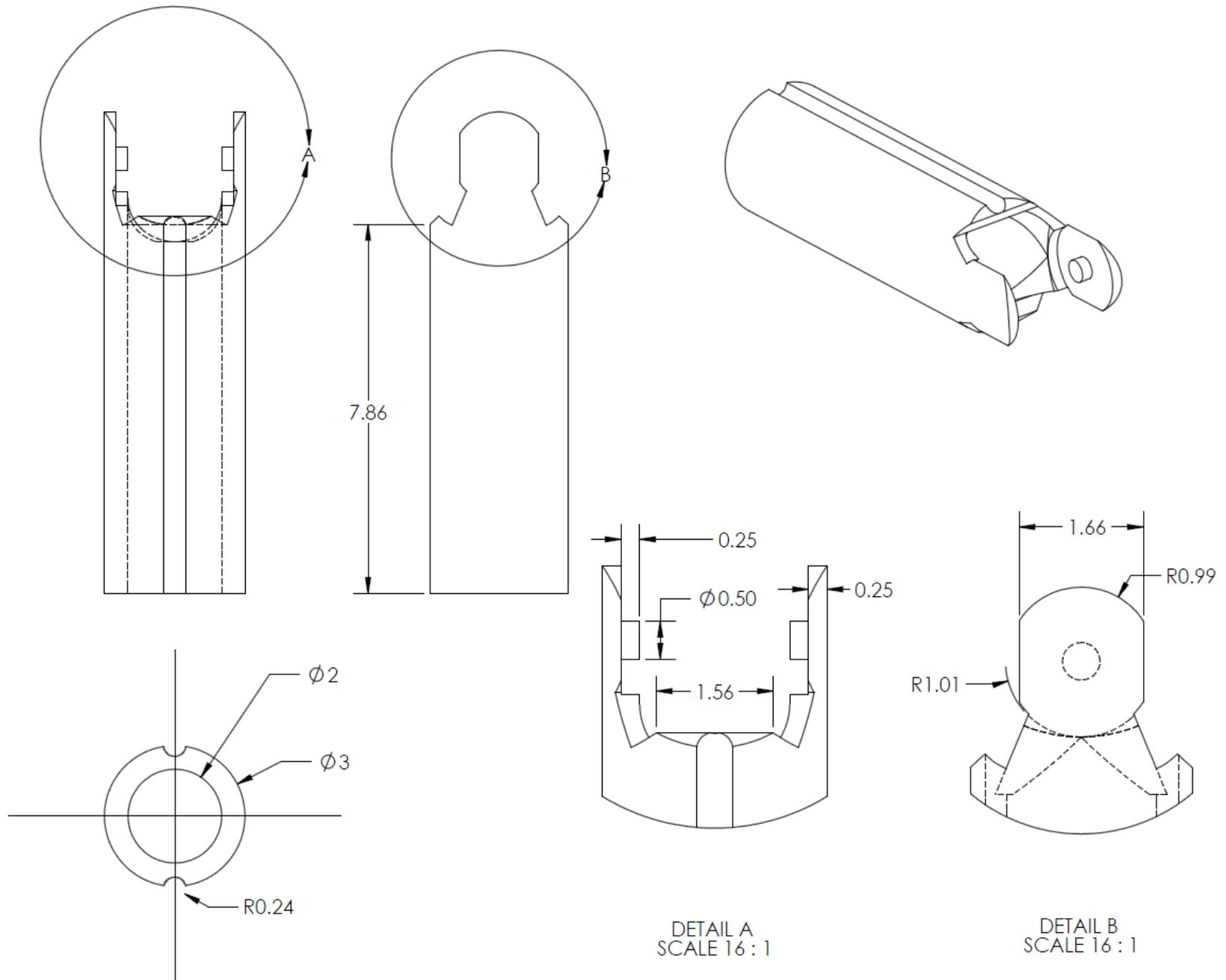
Figure 36. Bottom part of pin joint
