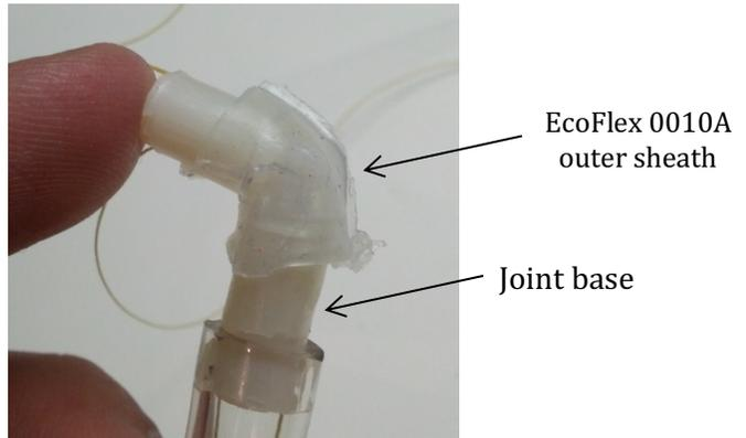
**Figure 29. 2:1 scale pin joint prototype**
