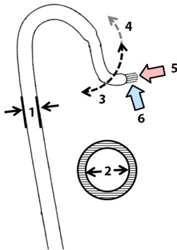
**Figure 6. Schematic of catheter wrist design parameters**
