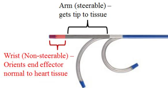
**Figure 3. Illustration of current steerable catheters, with ‘wrist’ region highlighted.**
