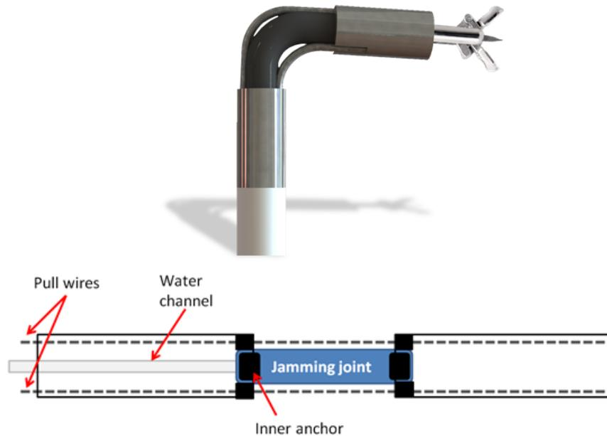
**Figure 18. CAD rendering of granular jamming joint design, with schematic**
