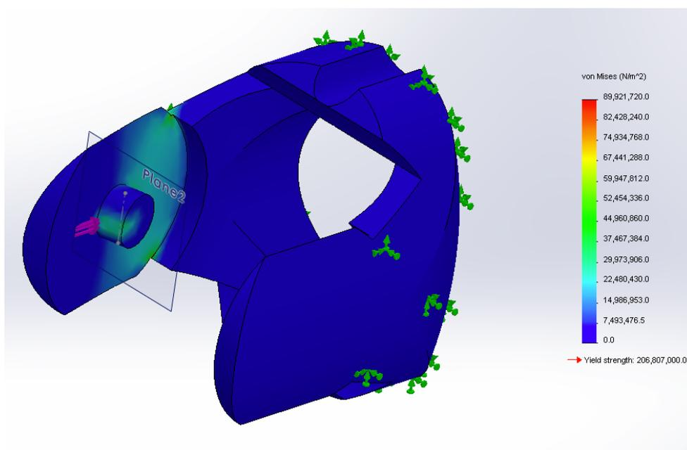
**Figure 12. CAD model of 1N force on pin in direction of arrow shown**
