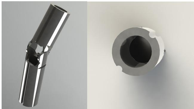
**Figure 28. Final prototype CAD model including catheter lumen**
