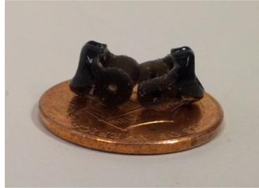
2:1 scale prototype with outer sheath and pull wires exposed
