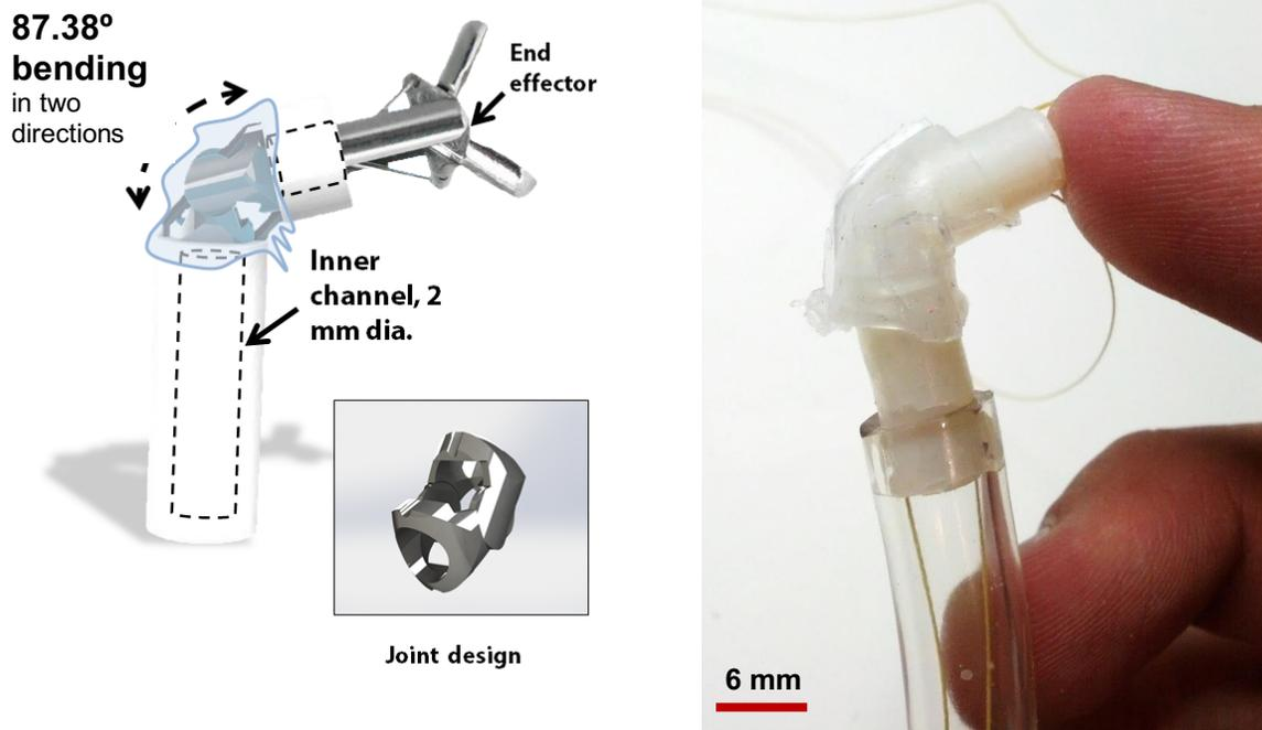
**Figure 7. CAD rendering of final pin joint design, with the joint highlighted (left); 2:1 scale prototype (right)**
