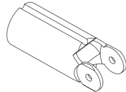
Figure 37. Top part of pin joint
