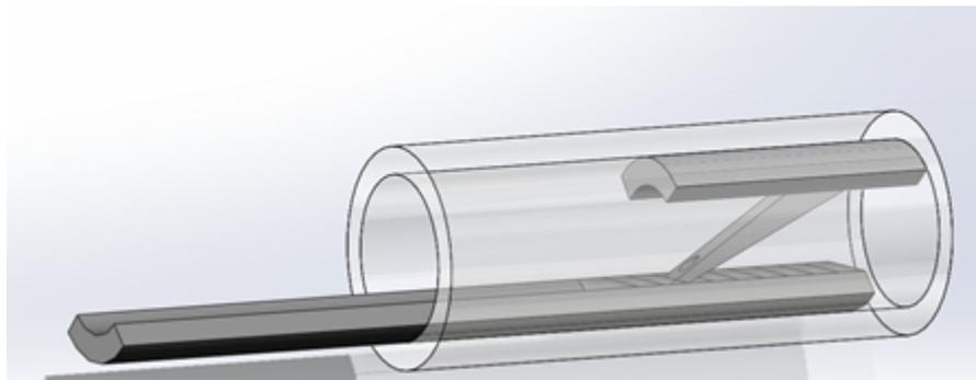
**Figure 23. CAD model of elastomeric catheter joint with locking mechanism**
