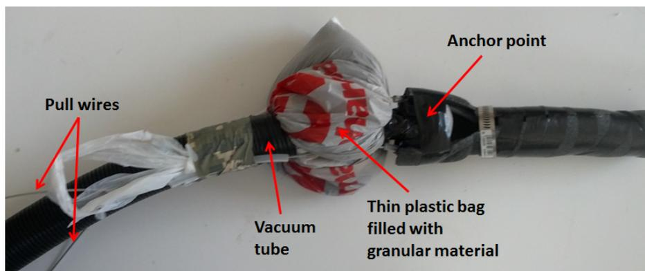
**Figure 19. Image of proof-of-concept jamming joint prototype**
